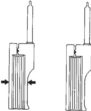
Fig. 13: Quick test to check bellows pump for leaks
