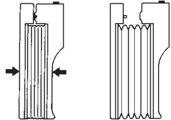
Fig. 14: Quick test to evaluate the suction capacity of the bellows pump
