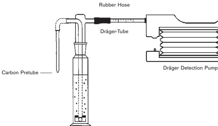
Fig. 33: Measurement system of the Dräger Liquid Extraction method
