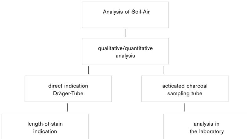
Fig. 34: Dräger-Tubes for soil air analysis
