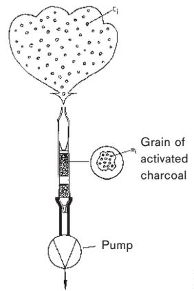
Fig. 41: Measurement principle of active sampling with Dräger activated charcoal tubes
