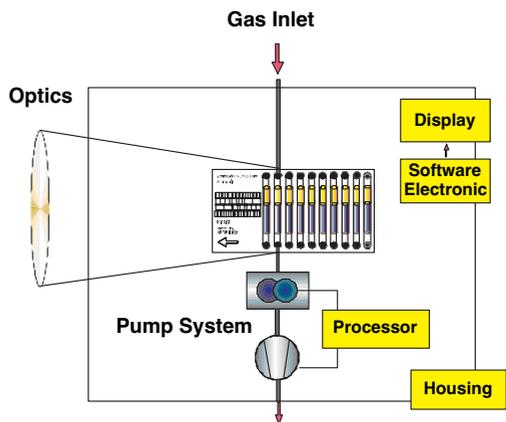
Flow Chart of the Measuring Principle
