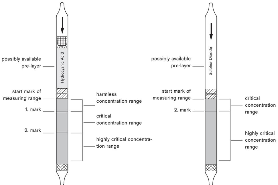
Fig. 30: Evaluation of the Dräger Simultaneous Test Sets
