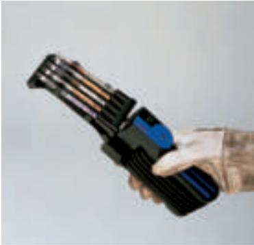
Fig. 31: Measuring with the Dräger Simultaneous Test-Set
