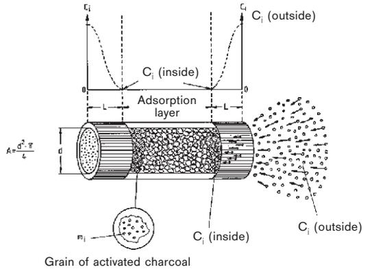
Fig. 43: Measurement principle of the Dräger Diffusion sampler ORSA
