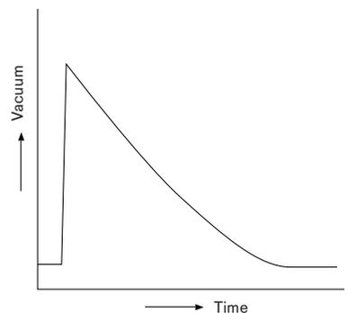
Fig. 9: Suction characteristic of a Dräger bellows pump
