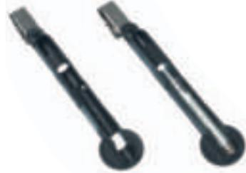
Fig. 7: Direct reading diffusion tube with holder
