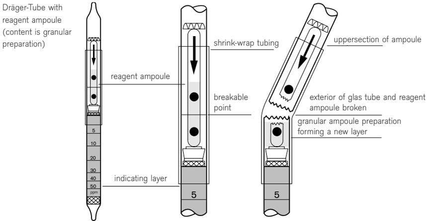
Fig. 19: Dräger-Tube with built-in reagent ampoule
