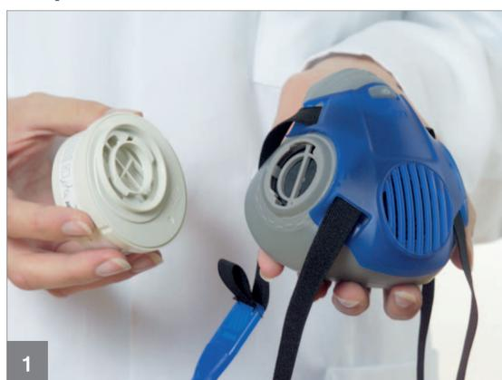
1 Attach the bayonet filters. The filter and mask body are marked to help you.
