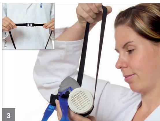
3 Place bottom straps over your head. With the Dräger X-plore® 3500 first connect the hooks on the neck strap (inset figure)
