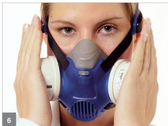
6 **Negative pressure test:** Seal both respiratory filters with your hands and breathe in until a negative pressure (suction) is generated. Hold your breath for a moment. The negative pressure should be maintained. If not readjust the face piece and adjust the straps or use a different size of mask. Repeat test until a successful seal check is met.
