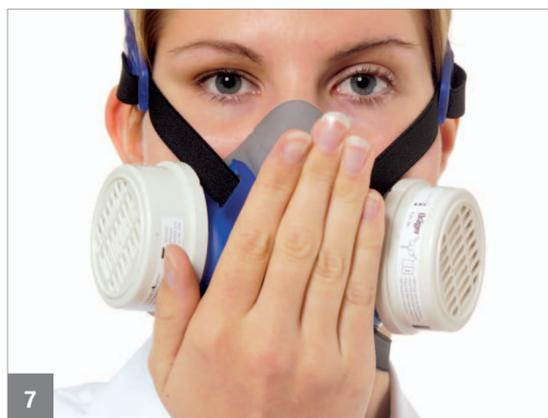
7 **Positive pressure test:** Seal the exhalation valve of half mask and exhale. The half mask will inflate slightly. If the exhaled air leaks out of the mask, readjust the face piece and adjust the straps or use a different mask size. Repeat test until a successful seal check is met.
