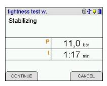
At the end of the stabilization period, the reduction of the test pressure is required.
