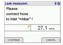
Now, purging is conducted for the connecting line and the measurement system for 40 seconds, to prevent falsifications of the measurement result. The gas is released from the gas connection between the pressure inlets for the mbar and bar sensors. At the same time, the flow rate is < 5 l/h. The stabilization phase automatically begins after purging.
