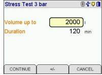
Connect the pipeline to be tested with the pressure inlet of the measuring device marked with "bar" using a pressure hose with a pneumatic quick coupling NW 5 and connect the external pump to the line via a valve.
