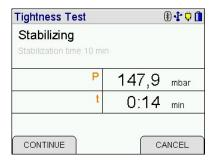
The pressure at the beginning of the measurement (P-Start), the current pressure or the pressure at the end of the measurement (P), the pressure difference (P-diff) and the already elapsed measurement period (t) are shown during and at the end of the measurement.
