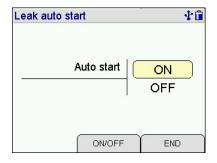
The measuring device recognizes a drop in pressure and automatically starts the leak rate measurement.
