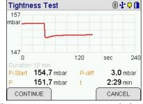
The start and stop values as well as the up to 20 intermediate measurements and the elapsed time were retained. These retained values can be stored and transferred to a PC at a later point in time. Measurement reports, which show the chronological sequence of the measurement in a diagram, can be printed using the PC200P software.
