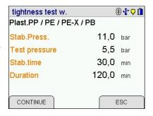
Connect the pressure sensor to the pipeline to be tested and start the measurement.
