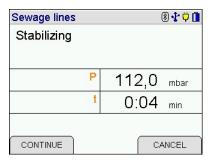
After the stabilization period has ended or using (CONTINUE), the instruction is given to reduce the pressure to the test pressure.
