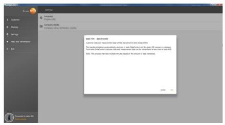
As soon as the testo 400 is connected via a USB cable to a computer, Connected to testo 400 – Synchronizing is displayed at bottom left.
