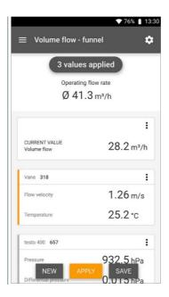
6 Apply: the current reading is applied.
