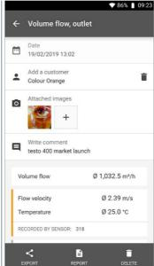
The calculated result of the measurement is displayed under the Customer data, Images and Comments.
