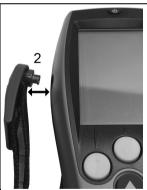
Engage the carrying strap clip in the fixing eyelets on the sides of the device. Note the guide groove, the strap must point "down" (2).
