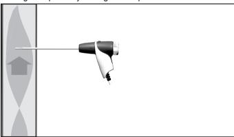
The tip of the probe must be in the hot spot of the flue gas flow.
