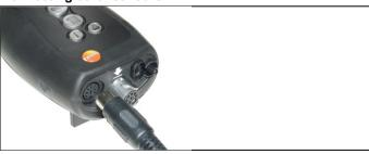
> Insert the connector plug of the probe into the probe socket.
