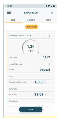
The measurement data is transferred to the testo Smart App and evaluated there.
