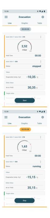
When the target values are reached, the evacuation and therefore also the pump are stopped automatically.
