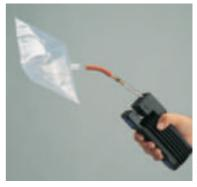
To conduct the test, exhaled air is blown through a resistance tube into a 1 L sampling bag. The air sample is drawn out of the sampling bag through a Dräger-Tube (calibrated in percent carboxy-hemoglobin) using the Dräger gas detector pump (Fig. 23).
