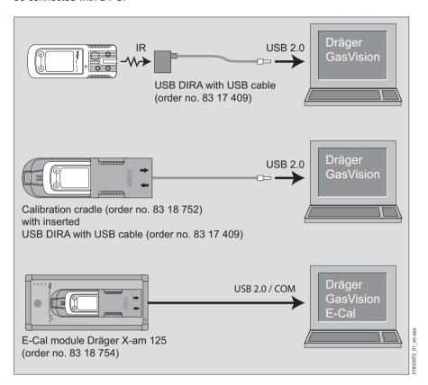
The installed PC software Dräger GasVision is used for reading and displaying the database.
