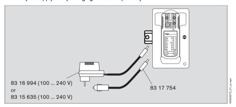
The charging process is carried out analogue to charging with the multiple charging station.
