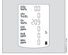
button calibration will be aborted. The channels will then indicate » n/a «. If only one sensor is taking part in the 1-button calibration, a calibration will be performed in each case when the  $\bigcirc$  key is pressed.
