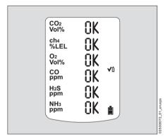
If the set bump test concentration is not reached within the specified time, the alarm mode is activated to indicate failure.
