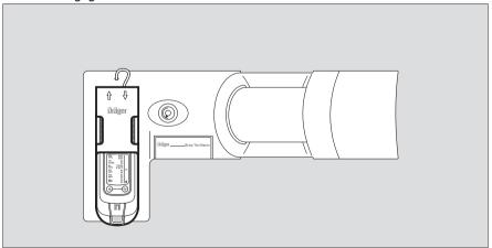
— The function test with gas is started automatically. The special symbol » √0 « (for bump test) flashes.
