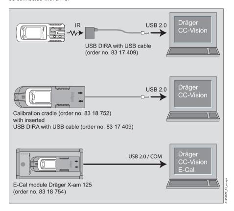
The installed PC software Dräger CC Vision is used for configuration.
